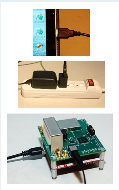
Figure 2 PulseGen Power Connections
